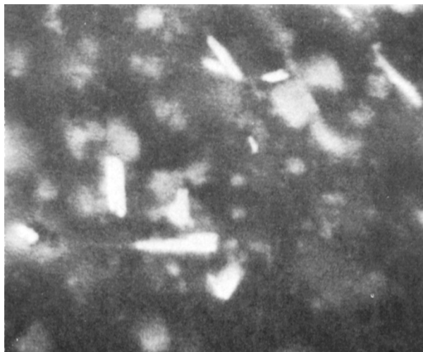
Fig. 9. Scanning electron micrograph of tribasic lead sulfate needles (5.0 phr) in the PVC formulation.
